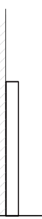
Throughout: Flat Profile Applied Wood Base 8"H X 1/2"W Returns @ Door Jams Locations W/ Tile Flooring 4" (+/-) Tile Base To Match Flooring
